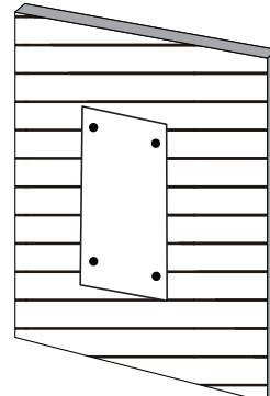
**NOTE:** When securing the hose reel assembly to plywood or dimensional wood, make sure the wood is thick enough to not only support the hose reel, but also the force required to extend and retract the air hose.
