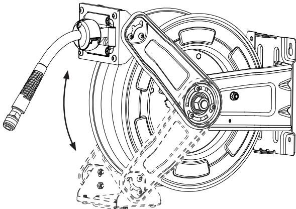
**NOTE:** If the desired angle is larger than 90 degrees, remove the 3 x screws **10** on each side and rotate the roller bracket **9** to the desired position. Replace the 3 x screws into the roller bracket and re-tighten.
