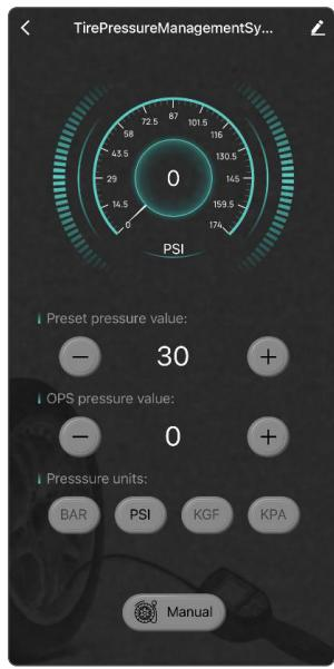
**3:** Once inflating and deflating is completed, the tyre inflator will beep to indicate completion. The app will switch to the completion interface.
