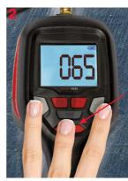
Whilst still holding down the "+" and "-" buttons also press the "on/off"button. The display will show one of the following codes: 05C, 05D, 05F, 060,061, 062, 063, 064,065, 066, 067, 068,069, 06A, 06B, 06C.
