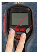
To begin ensure that the inflator is turned off and the screen is blank. To begin, hold down the "+" and "-" buttons at the same time
