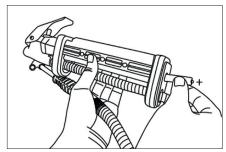
Slide the batteries into the inflator with the positive end facing out of the inflator
