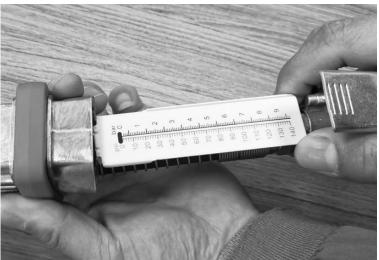
**STEP 3** Loosen the two nuts with a spanner to adjust the scale back to zero.
