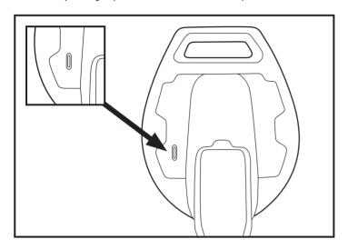
2. When battery is charged, remove USB-C cable from port.
